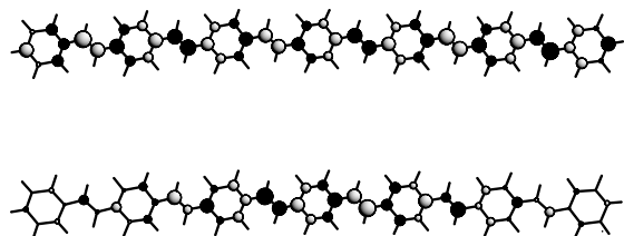
Fig. 5. LUMO of 7PV 2+ for the SCC-DFTB (upper panel) and DFTB (lower panel) methods. The size of the circles is proportional to the p_z wavefunction coefficient of the respective atom, the shading indicates the sign.
